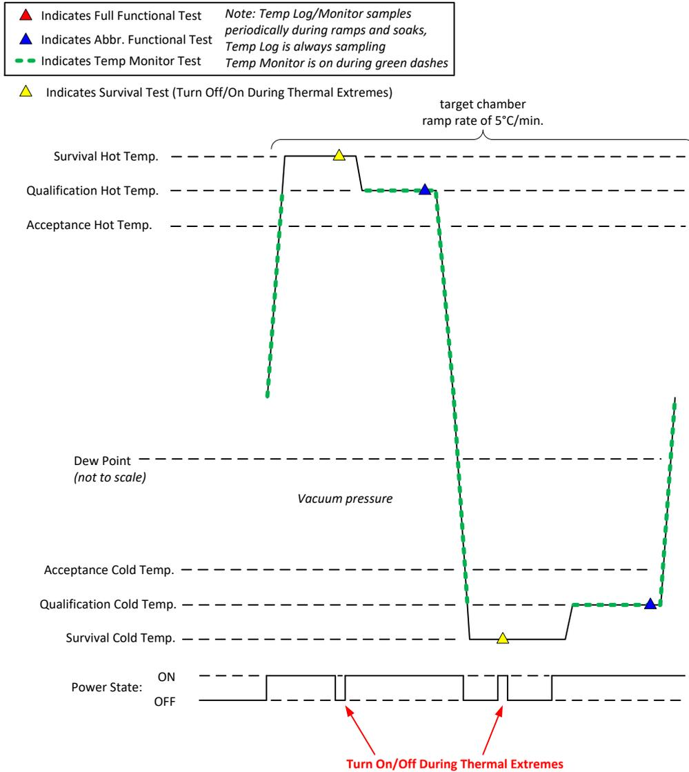
**Figure: Typical Thermal Vacuum Cycle**
