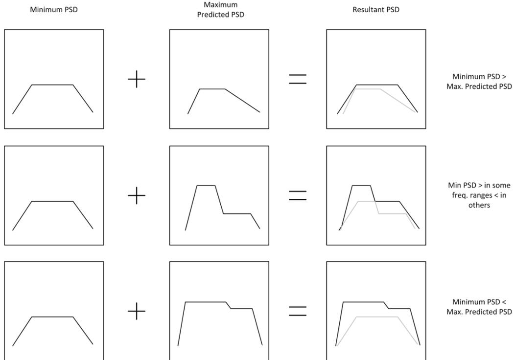
**Figure: Applied Random Vibration Spectrum Envelope**
