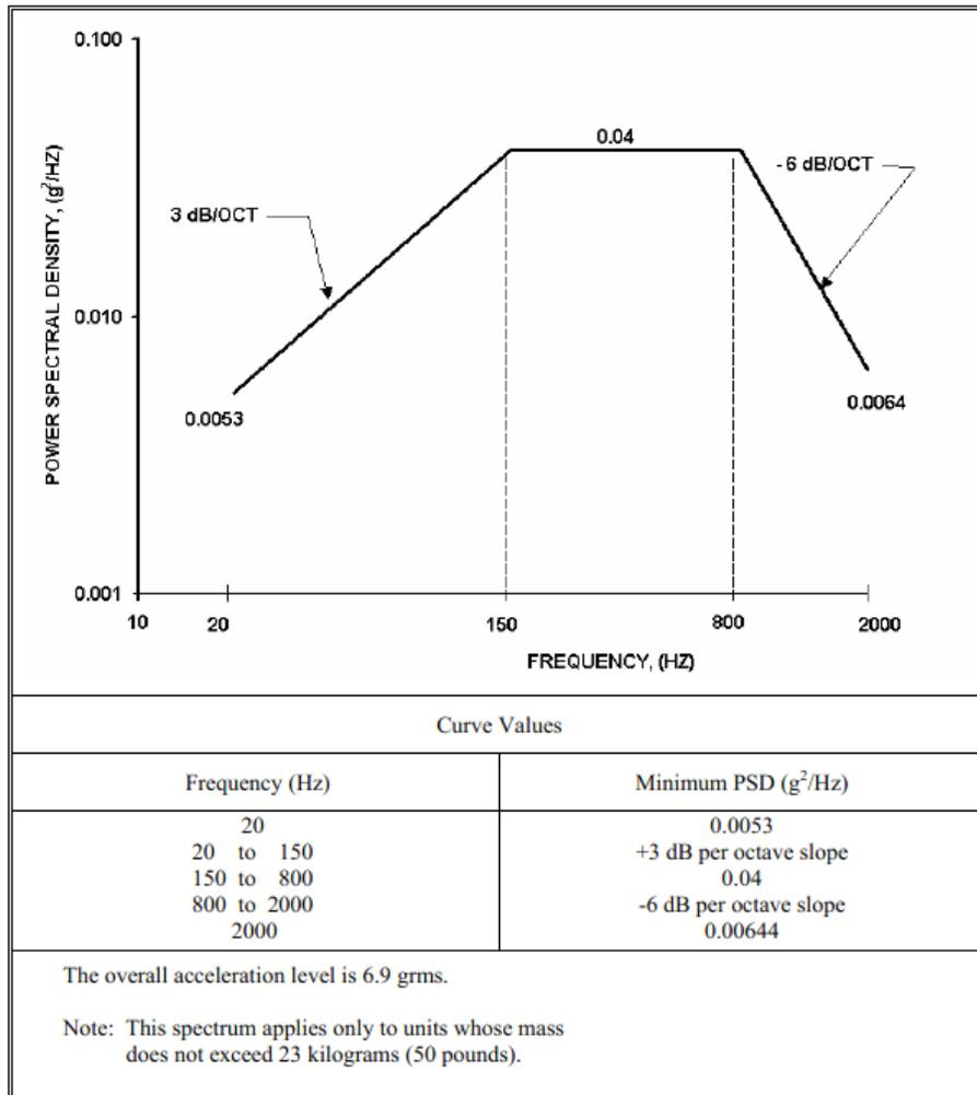
**Figure: Module Acceptance Workmanship Random Vibration Spectrum**
